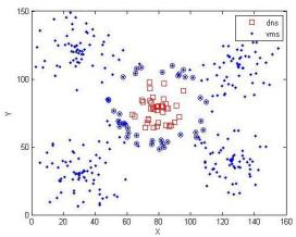
Figure.3 The VM placement result of VSMR. The distribution of VMs is intensive when they are far from data nodes and sparse when they are closer.
