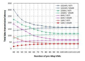
Figure.4 VSTI vs VSMR in minimizing total data transmission latency for different number of pre-Map VMs and 40 data nodes.
