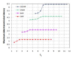
Figure.7 The maximum data transmission latency for different threshold  $t_1$  using VSMR
