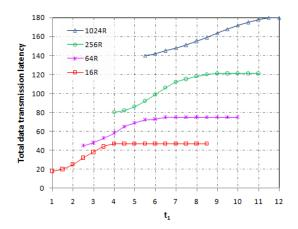
Figure.6 The total data transmission latency for different threshold  $t_1$  using VSMR
