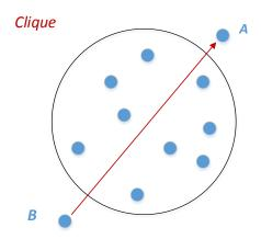
Figure.1 Both VM *A* and *B* satisfy the constraint of clique selection. However, only one of them will be added into the clique, since the latency between them exceeds the threshold.
